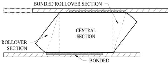
*This technology is aimed at hazard mitigation of regular low-rise buildings in high seismic*
